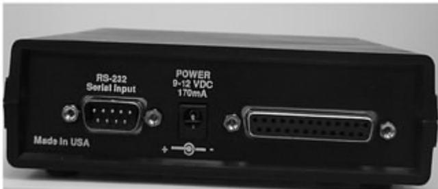
Figure 1a. P2RS Parallel to Serise Converter
